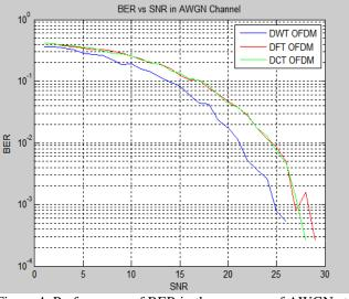
Figure 4: Performance of BER in the presence of AWGN at different SNR.
