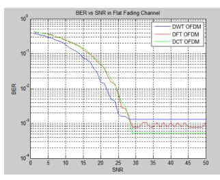
Figure 5: Performance of BER over Rayleigh flat fading channel in the presence of AWGN.
