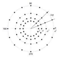
Figure 2: 64-DAPSK constellation diagram.
