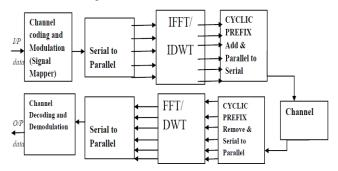
Figure 1: Block diagram of a OFDM system.
